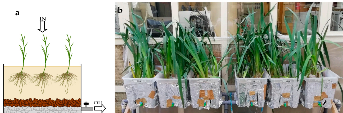
Figure S1. (a) Schematic representation of CW microcosm; (b) Picture of real CWs microcosms with T. latifolia . The wastewater is changed every 15 days.
