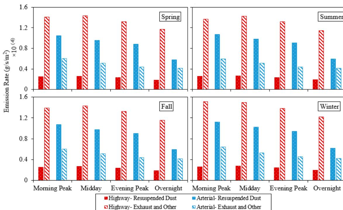
Figure 2. Predicted fine particulate matter (PM<sub>2.5</sub>) emission rates.
