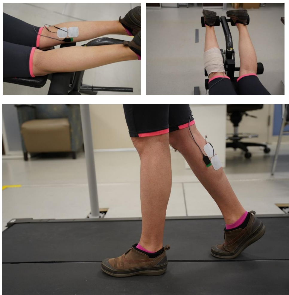
Figure 4. (Top Left) mTrigger and DELSYS electrode placement. Electrodes were placed on the medial gastrocnemius with DELSYS electrode always medial to mTrigger electrodes. (Top Right) A flex wrap was used to minimize electrode movement and wired movement. Wraps were removed to illustrate electrodes in different positions and different data collection settings. (Bottom) Participant in a push-off position walking on a treadmill.
