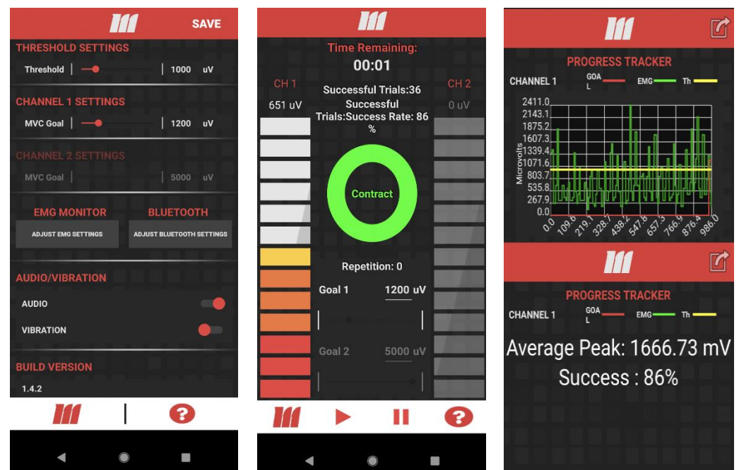
Figure 3. (Left) The setting panel for the mTrigger phone app. The threshold and goal are set on this screen. Additionally, audio, and haptic (‘vibration’) feedback can be turned on or turned off. (Middle) This panel is displayed during training. Near the top, time remaining as well as the number of successful trials and overall success rate is shown for the trial. The red to gray bar graph on the left side indicates progress towards a force goal for Channel 1. (Top Right) This shows the tracking panel. This panel is used to display the session data. The square button with the arrow is used to upload the data to Google Cloud. (Bottom Right) This is displayed when clicking on the tracked data (Top right), which shows the average peak muscle activity for the duration of trial and the success rate. This average number can be used in an initial trial to detect and set the initial threshold and subsequent activation goals. Success rate can be used as an outcome measure and additionally to make sure participants meet the increased goal at a minimum rate.
