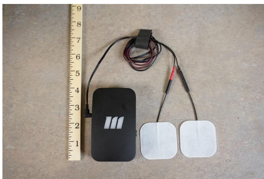
Figure 1. mTrigger device and disposable electrodes. This is a 2-channel system, but in this study, only 1 channel was used.
