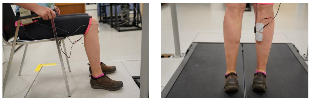
Figure 2. (Left): Drift test—participants spent 5 min in a seated position with knees flexed at 90 degrees and were instructed not to move. (Right): Lag test—participants performed heel rises to match a metronome at 45, 60, 75, and 90 BPM for 30 s.
