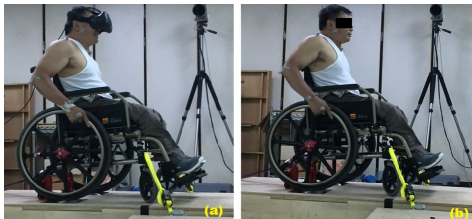
Figure 1. Participant pushed the wheelchair with (a) and without HMD (b) on a stationary ergometer.
