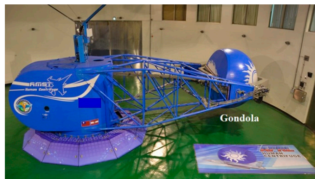
Figure 3. Human centrifuge in APRL.
