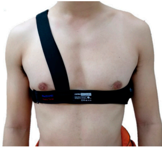
Figure 2. BioHarness 3.0 module attached to chest and shoulder straps.
