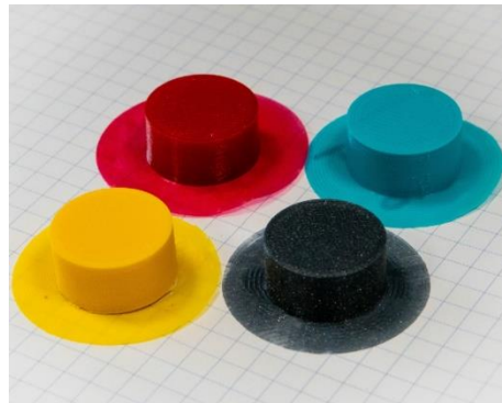
Figure 2. Example of printed samples with a detachable brim structure, yellow—ABS, red—TPU, blue—PET-G, grey—PLA.
