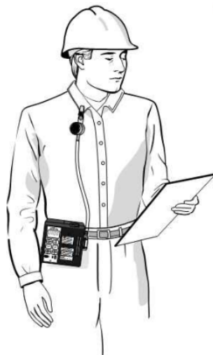
Figure 6. IOM sampler and pump on worker
