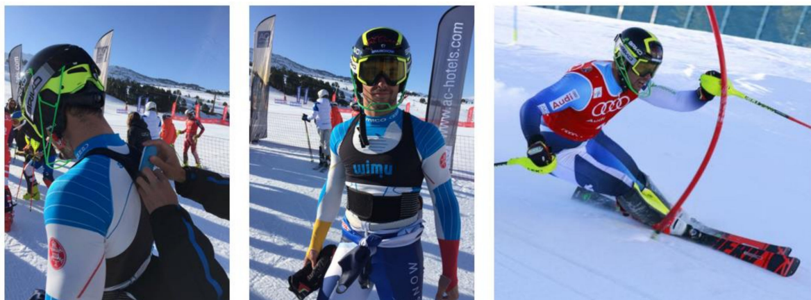
Figure 1. The placement of the Global Navigation Satellite Systems (GNSS) device on the vest on the skier.
