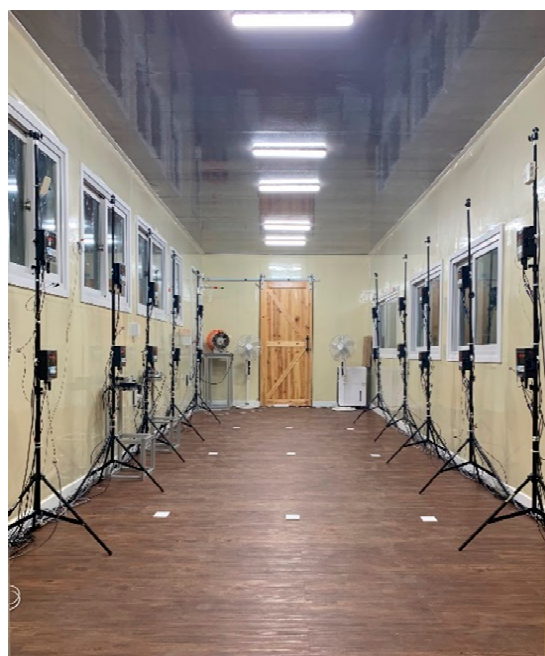
Figure 1. Inside the classroom chamber (Note: cube-shaped devices on the poles are simple particulate matter (PM) measurement devices but they were not used in this study).
