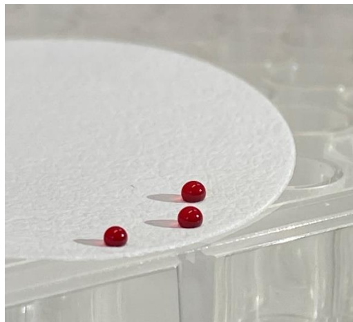
Figure 3. A 2 \mu\text{L} blood drop deposited on a PTFE filter; the drop remained spherical even after drying.
