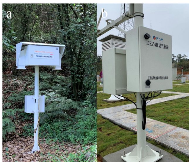
Figure 2. Meteorological observation system, including; (a) FR500 negative oxygen ion monitor, and (b) DZZ4 automatic meteorological station.
