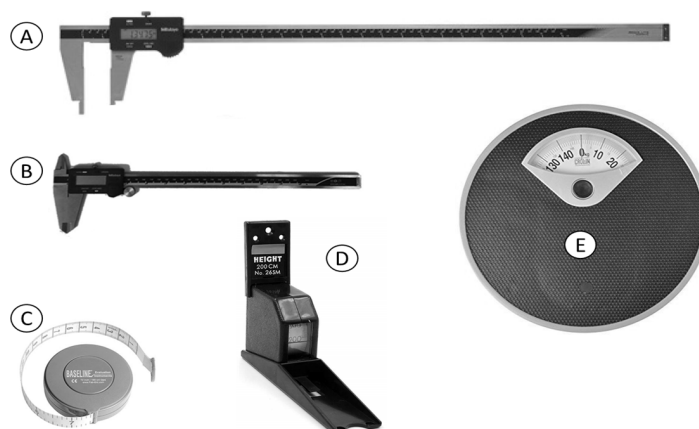
Figure 2. Measuring instruments used in the survey. Note: (A) larger sliding caliper; (B) small sliding caliper; (C) plastic measuring tape; (D) stadiometer and (E) weighing scale.
