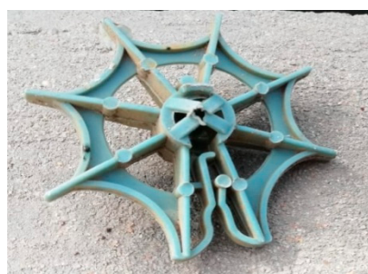
Figure 2. The star-shaped plastic media used as submerged biofilter.
