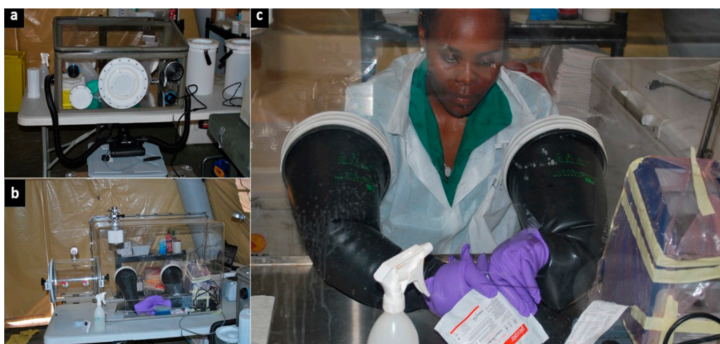
Figure 2. Two portable negative-pressure gloveboxes. (a) The smaller glovebox was used for inactive Ebola virus in patient samples, perform malaria tests, and monitor biochemical parameters with the handheld blood analyser. (b,c) The larger glovebox was used to monitor biochemical parameters with the Piccolo Xpress and to prepare the Biofire Filmarray cassette for Ebola diagnostics (not shown).
