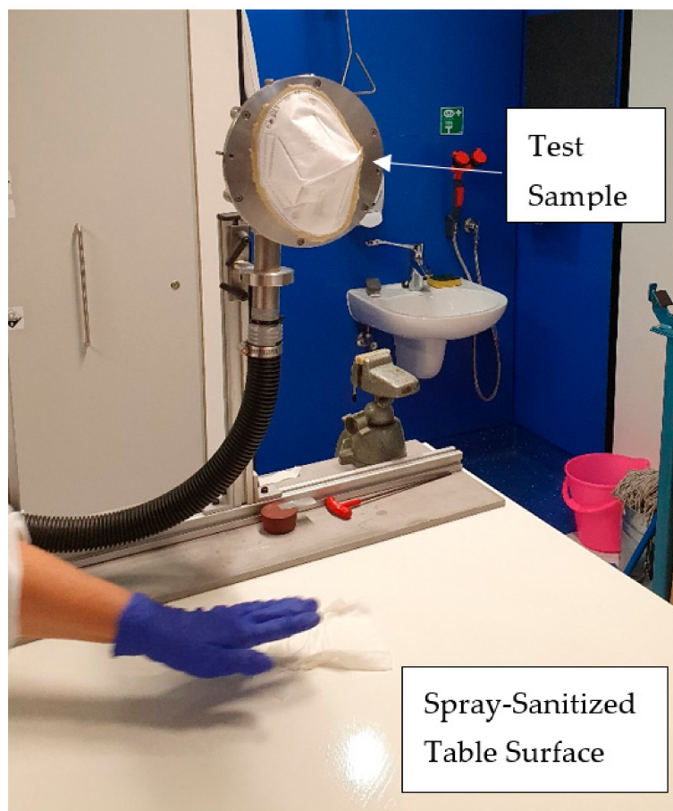
Figure 3. Experimental set up for exposing respirator test samples to alcoholic vapors (IPA) emitted by the process of spraying alcohol solution on a table surface followed by wiping with a paper towel.
