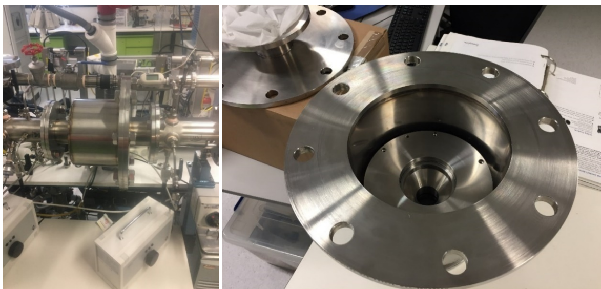
Figure S3. Filter test chamber used for ‘whole-mask MPPS’ testing with sampling provisions for pressure drop and particle concentration measurement up- and down-stream of the mask sample (left), as well as mounting provisions inside the test chamber (right).
