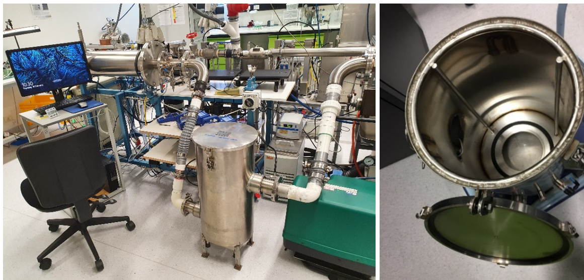
Figure S2. Filter test equipment used for 'whole-mask screening' tests, showing on the right the interior of the 15L test chamber.
