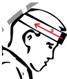
Figure 3. The Wiva ® Science motion sensor mounted to the head to measure acceleration, “a”. The sense of the vector “a” presented in the figures corresponds to its positive values; the opposite direction would correspond to negative values, mainly obtained in group B.
