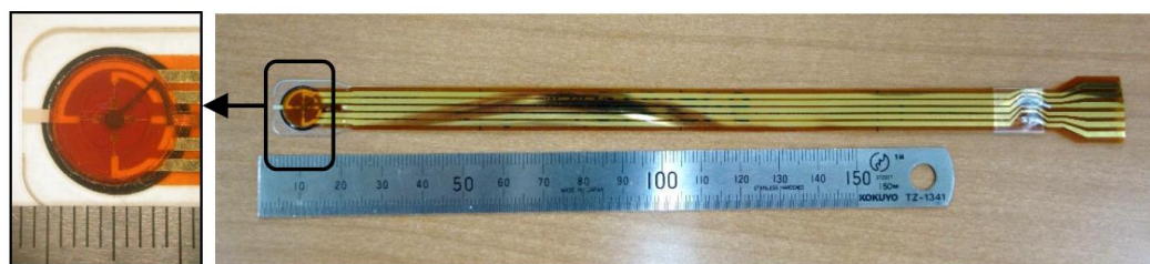
Figure 1. Tri-axis load sensor. Overview of the tri-axis load sensor.
