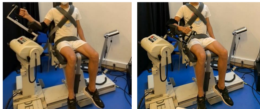
Figure 2. Player positioning during the shoulder internal and external rotations performed on the isokinetic dynamometer (left and right panels, respectively).
