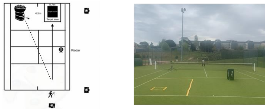
Figure 3. Experiments conducted on the tennis court and the respective ball machine, marking tapes, video cameras, and radar (left and right panels).
