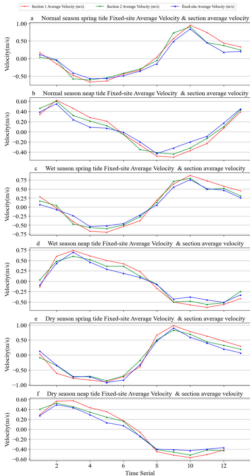
Figure 6. Process curve of fixed-site buoy vertical average velocity and section average velocity. (a) Normal season spring tide average velocity & section average velocity of the fixed-site, (b) Normal season neap tide average velocity & section average velocity of the fixed-site, (c) Wet season spring tide average velocity & section average velocity of the fixed-site, (d) Wet season neap tide average velocity & section average velocity of the fixed-site, (e) Dry season spring tide average velocity & section average velocity of the fixed-site, (f) Dry season neap tide average velocity & section average velocity of the fixed-site.
