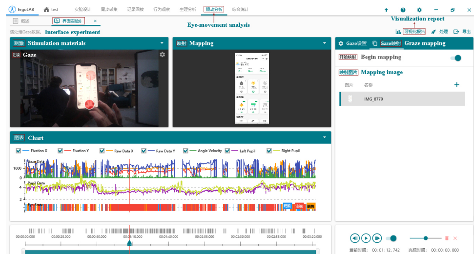
Figure 2. The platform for experimental field runs. It consists of three main windows: live video and eye movement data filmed real-time, real-time mapping of stimulus materials, and real-time monitoring of physiological sensor data.
