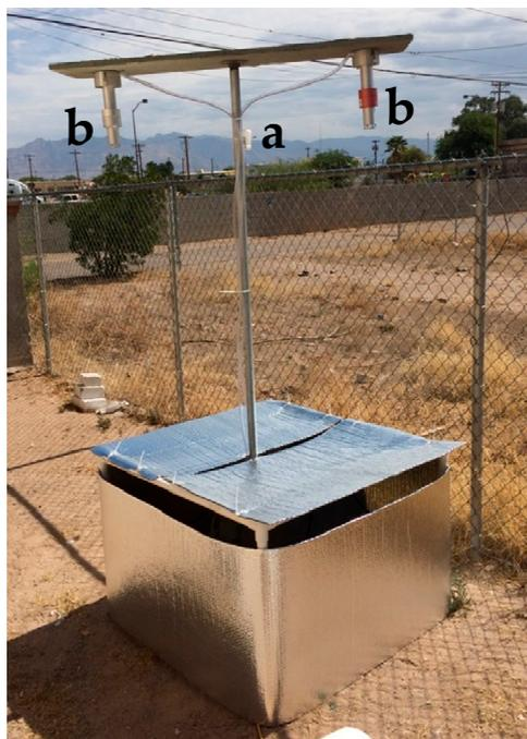
**Figure 2.** A typical sampler setup for  $\text{NO}_2$ ,  $\text{NO}_x$ ,  $\text{PM}_{2.5}$ , and  $\text{PM}_{10}$ . The Ogawa Badge Sampler (a) is attached near the top of the central post, while Harvard impactors hang, inlet down, from each end of the horizontal plank (b). Leland Legacy pumps are in a pump case concealed by UV-reflective foil insulation.
