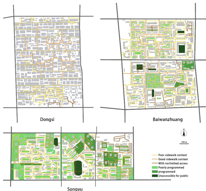
Figure 4. Sidewalks and green structures in the neighborhoods.
