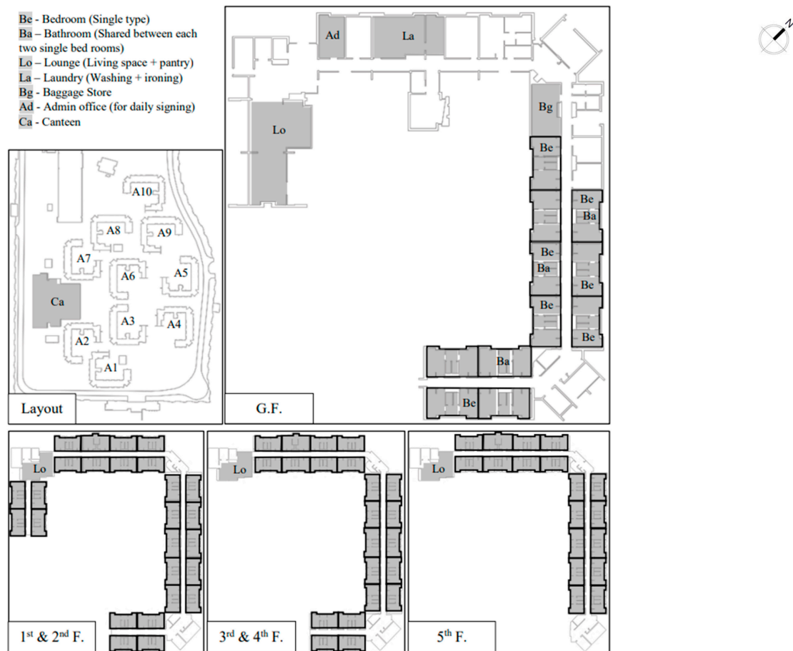
Figure A4. Typical ground and 1st to 5th floor layouts of the New Campus hostel, Building-A4.
