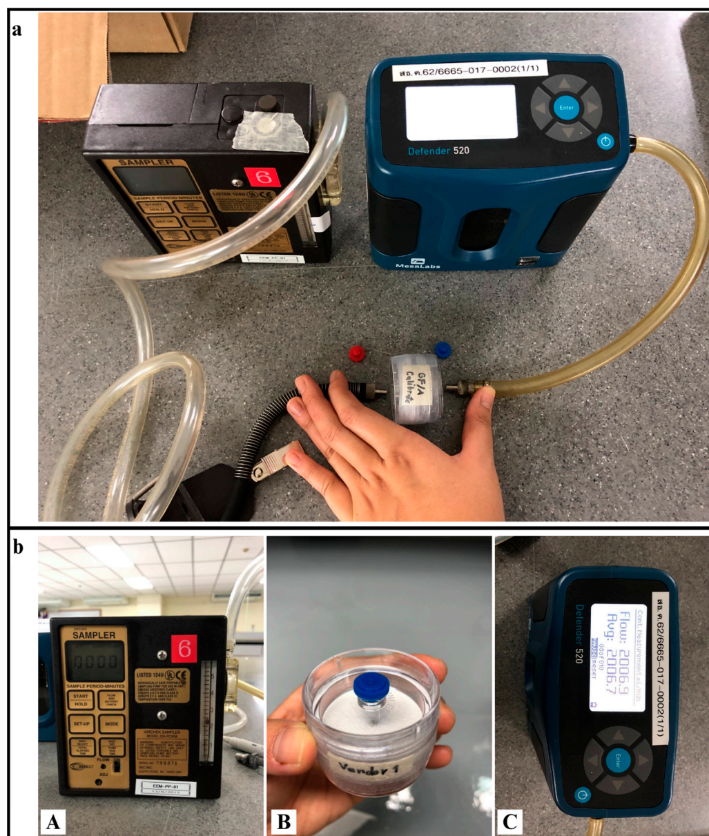
Figure 2. (a) The personal air sampler; (b) component of the personal air sampler: (A) personal air sampling pump; (B) GF/A pad placed in cassette filter; (C) pump calibration equipment.
