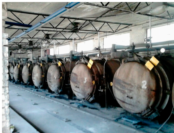
Figure 7. View of the production hall with autoclaves.
