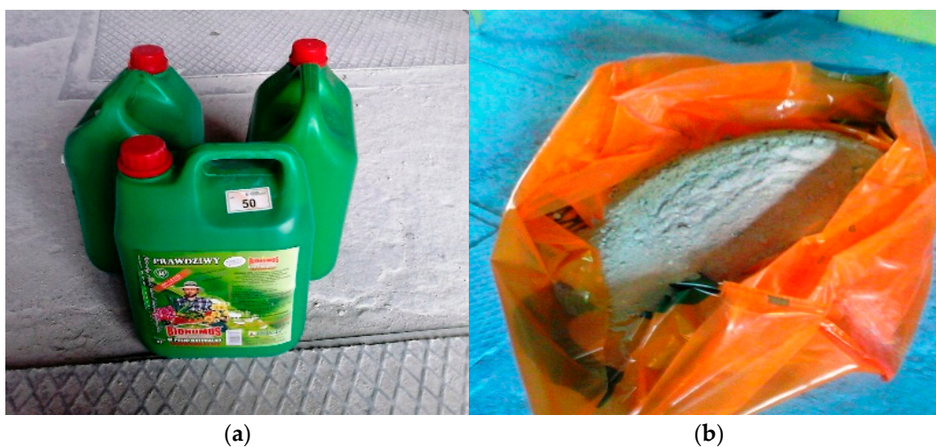
Figure 6. Substrates for the production of lime–sand brick modified with biohumus (biohumus in liquid form and quartz sand): (a) mix modifier used in the lime–sand mixture; and (b) modified sand–lime mixture.
