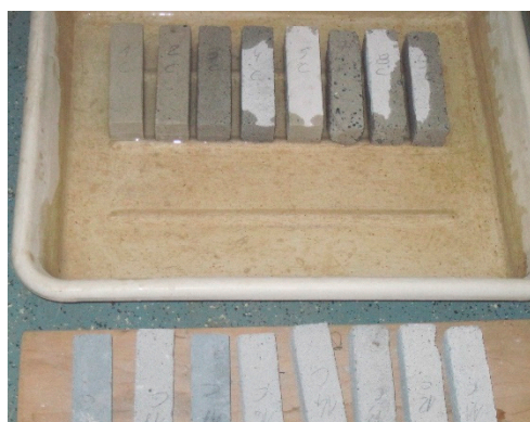
Figure 12. Study of the absorption caused by capillary rising of modified sand–lime products.
