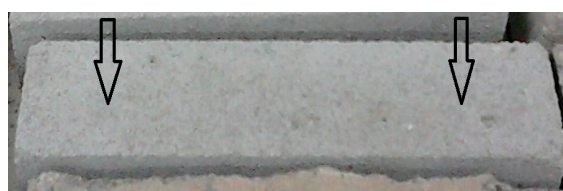
Figure 9. Compressive strength test of a laboratory beam with dimensions of 4 \times 4 \times 16 cm.
