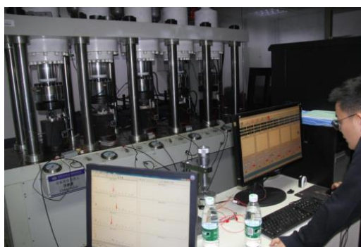
Figure 5. The five-link creep experiment system.
