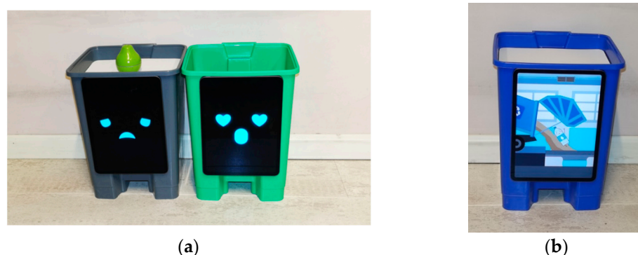
Figure 4. Expressive reactions of the designed intelligent trash can system toy. The toy displayed different expressions to distinguish whether users threw the garbage into the wrong trash can or not (a). The garbage thrown in the trash was displayed in the form of cute cartoons on the monitor (b).
