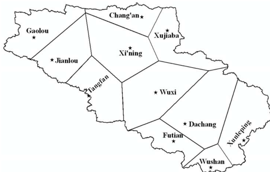
Figure 7. Spatial distribution of raingauges and associated Thiessen polygons in the Daning River watershed.
