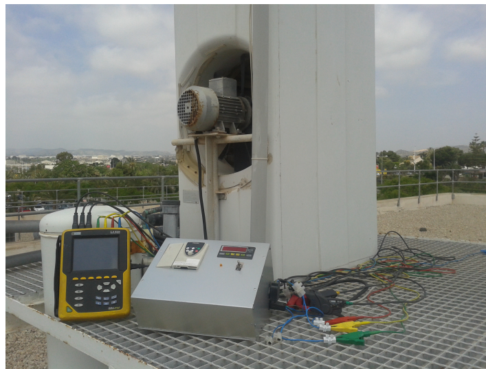
Figure 3. Power analyzer and frequency shifter at the pilot plant.
