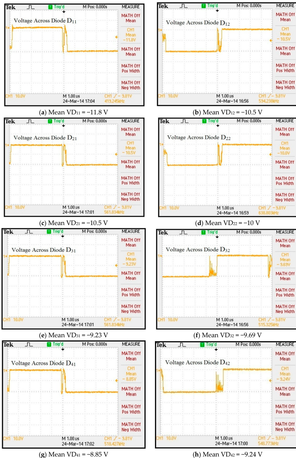
Figure 27. Voltage across diodes (a) D_{11} (b) D_{12} (c) D_{21} (d) D_{22} (e) D_{31} (f) D_{32} (g) D_{41} (h) D_{42} .
