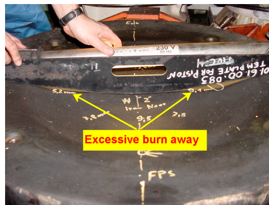
Figure 1. Burn away on spare piston crown.
