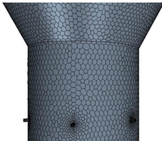
Figure 2. Meshed gasifier geometry and customized mesh at air inlets.
