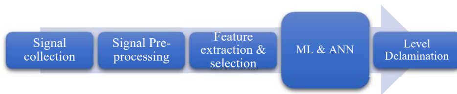
Figure 1. Process for determining the level of delamination in the Wind Turbine Blades (WTB). Machine Learning (ML); Artificial Neural Networks (ANN).
