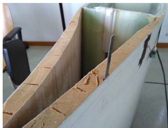
Figure 6. Placement of sensor and delamination.
