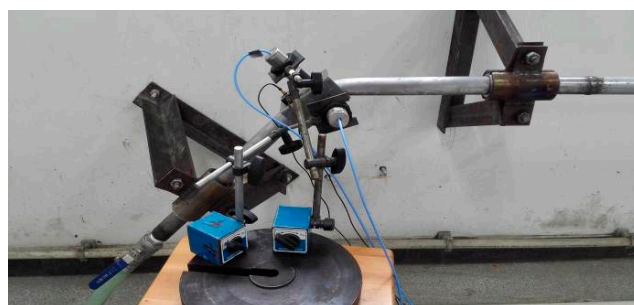
Figure 10. Physical map of pipe vibration test device and stress test device in elbow section.
