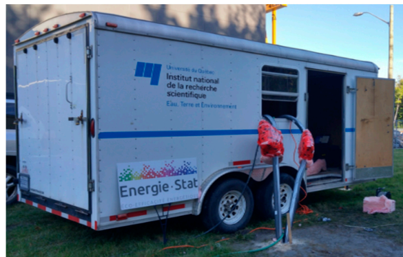
Figure 3. Experimental setup for the TRTs presented in this work (picture taken from [18]). Temperature sensors are located and the pipe inlet and outlet with red connections. Reproduced with permission from INRS [18], 2016).
