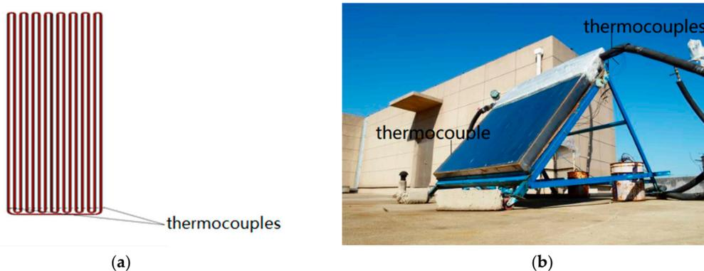
**Figure 1.** The design of oscillating heat pipe with 16 elbows and thermocouples (a), and the outdoor experimental facility of the solar collector of the oscillating heat pipe in a flat-plate structure (b).
