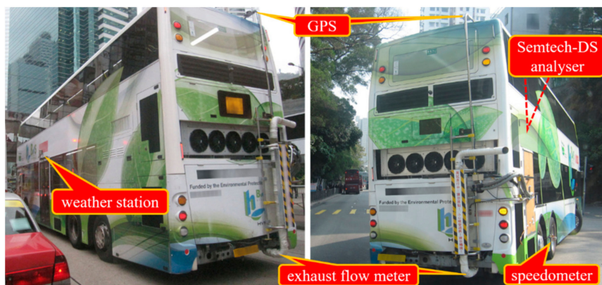
Figure 1. Euro VI diesel-hybrid bus during trials in the streets of Hong Kong. GPS: global positioning system; Semtech-DS analyser (Sensors, Inc., Saline, MI, USA).
