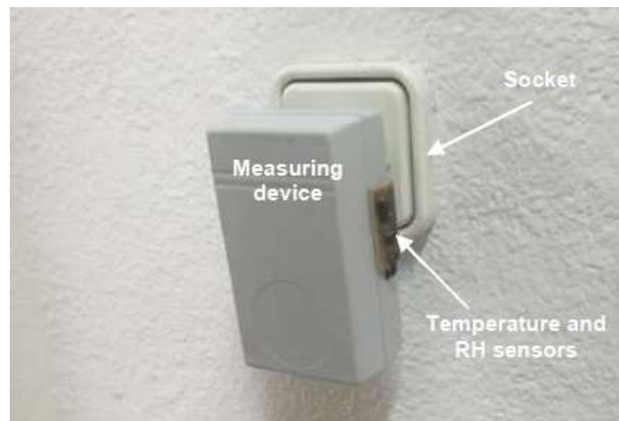
Figure 5. Measuring device installed in a socket outlet of the house.
