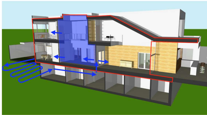
Figure 12. Layout of the LEGE system in Casa Zaranda.
