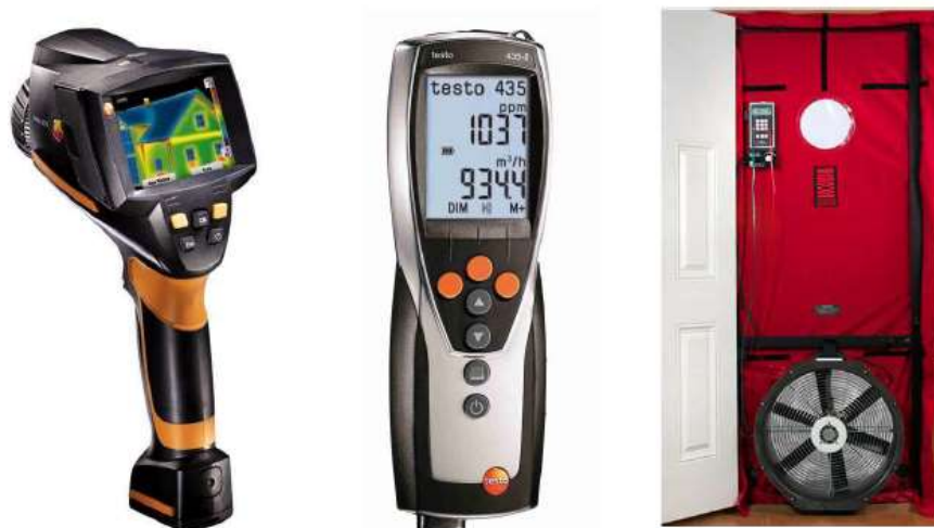
Figure 1. The thermal imaging camera, the transmittance meter, and the blower door test device.
