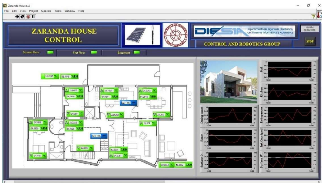
Figure 13. Location of sensors (T, RH, and CO 2 ) on the ground floor.
