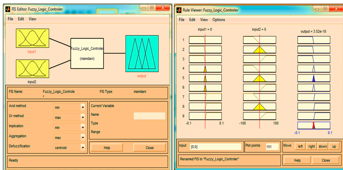
Figure 11. Max-min composition for the calculation of \Delta D output.
