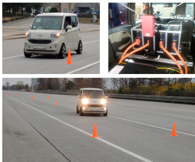
Figure 17. Slalom test and measuring sensor.
