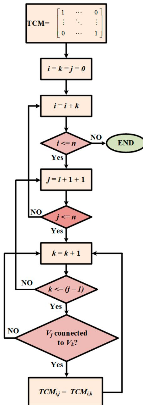
Figure 5. Flowchart for  $[TCM]$  calculation.
