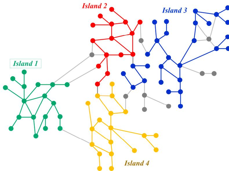
Figure 2. A Power system with four islands.
