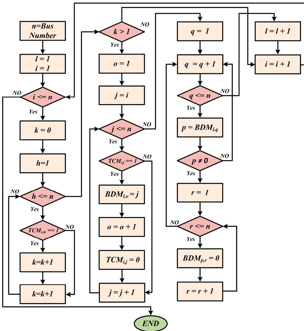
Figure 6. Procedure to extract subsections and bus-bars.
