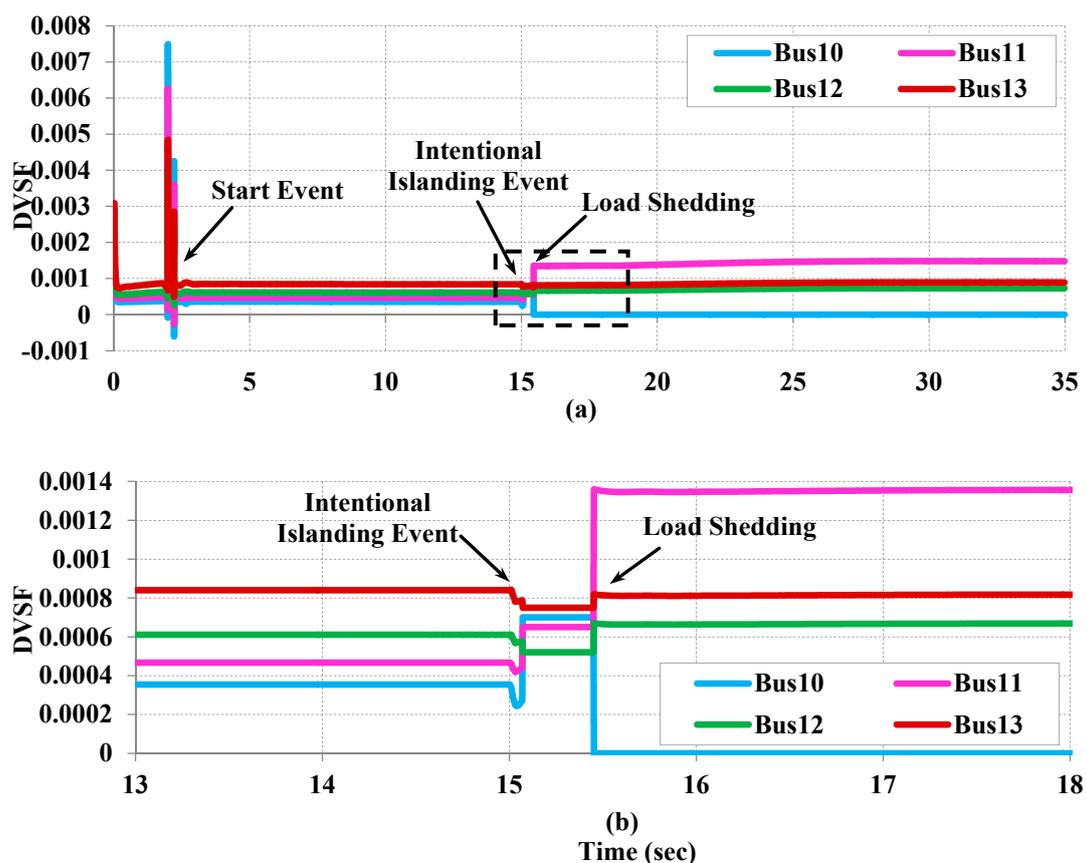
**Figure 16.** Dynamic voltage sensitivity factor (a) full window of DVSF for bus-bars in the island-2, (b) Expanded window for DVSF during ‘intentional islanding event’ and ‘load shedding’.
