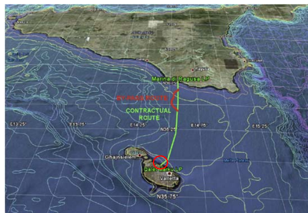
Figure 2. Sicily–Malta electrical connection (operating) [28]. Maghtab station is indicated by the red circle.
