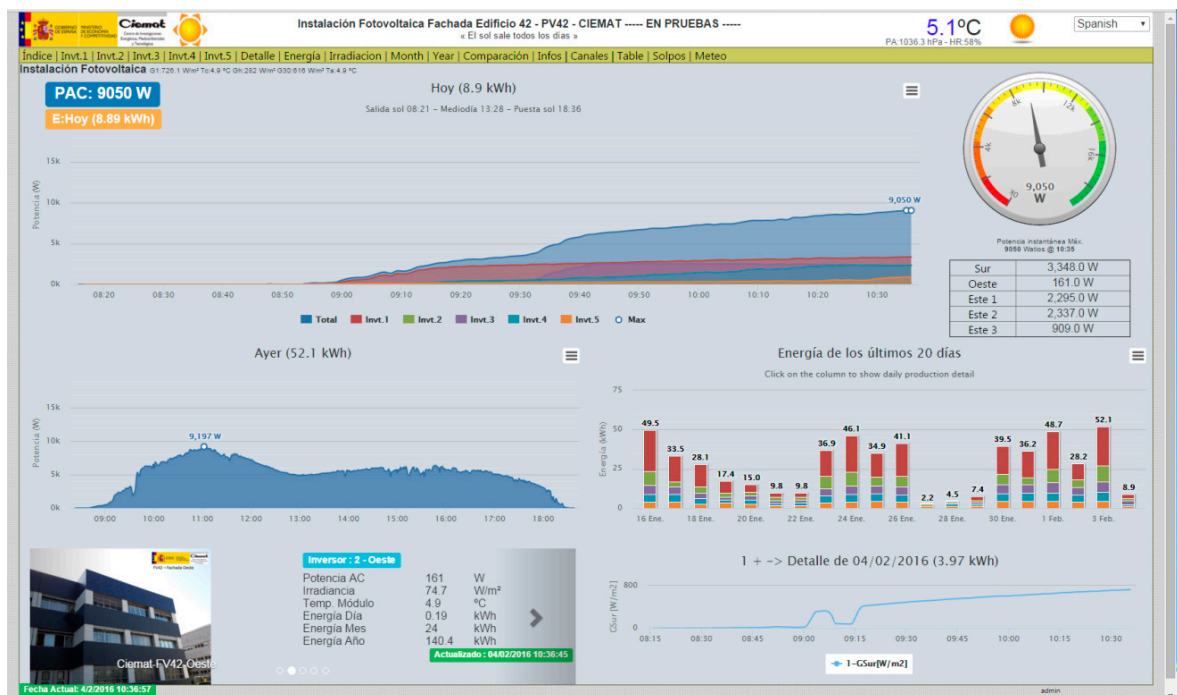
Figure 6. Real-time monitoring of the electrical variables of the grid-connected photovoltaic installation.
