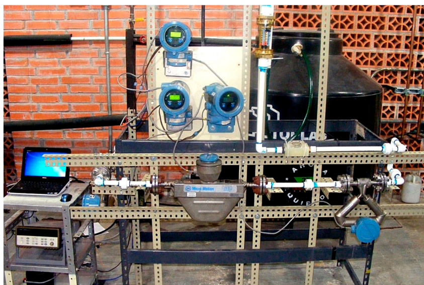
Figure A1. Calibration work of Coriolis type flow meters.
