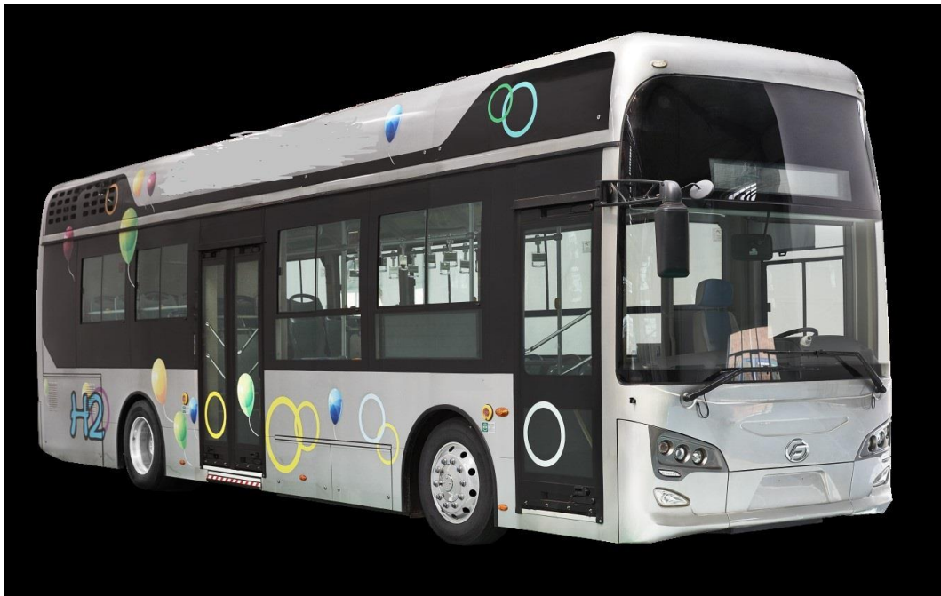
Figure 2. The 11 m Hydrogen fuel cell battery hybrid bus built by Feichi (Allenbus) in the new Yunfu factory. 11 of these were tested to provide the results given here.
