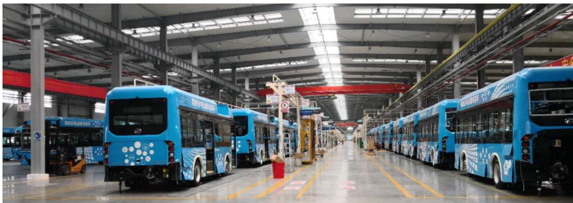
Figure 1. Production line of 300 hydrogen fuel cell battery 8.5 m buses in the new Feichi factory Yunfu in November 2017.
