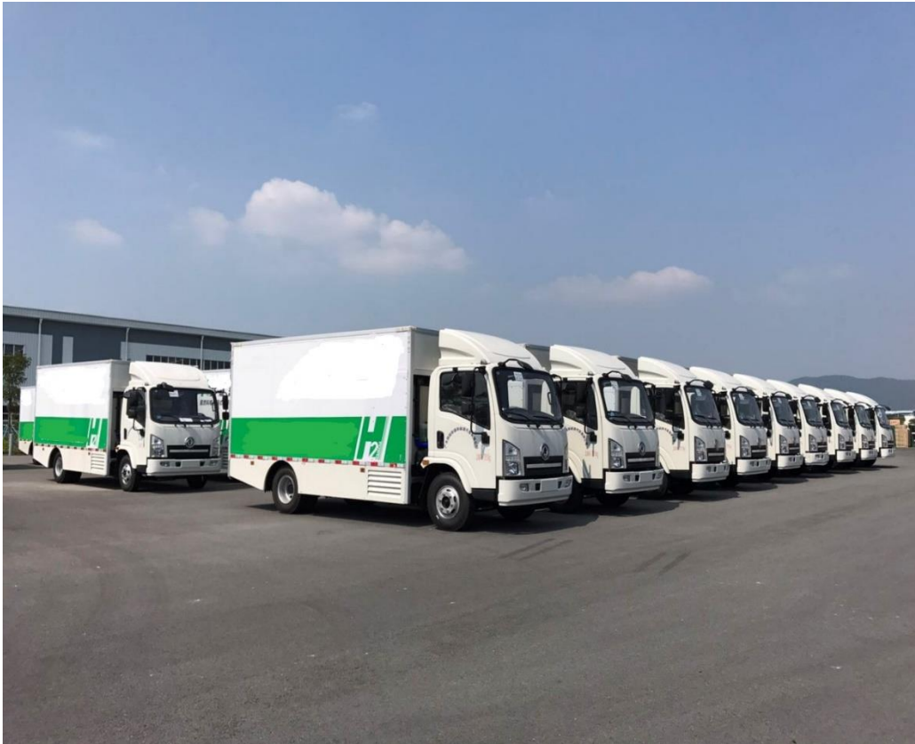
Figure 8. Hydrogen-Fuel Cell-battery delivery trucks built in China in 2017 to 2018 with 30 kW Ballard engines manufactured in Yunfu [15].
