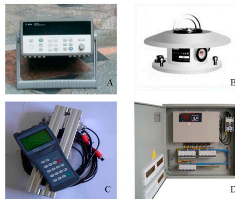
Figure 5. Measuring instruments. (A) HP34970A data collector; (B) TBQ-2 pyranometer; (C) YB-70H hand-held ultrasonic flowmeter; (D) DF-type centralized electric energy meter.
