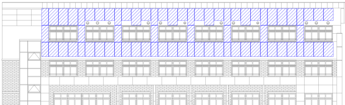
Figure 1. Air-type building integrated photovoltaic/thermal (BIPVT) collector on the demonstration building.
