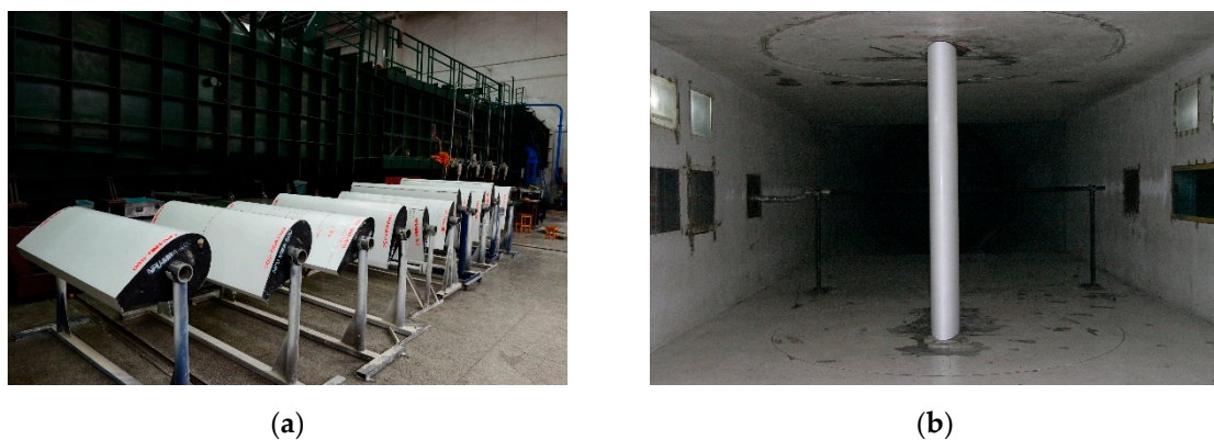
Figure 3. Experimental test of NPU-MWA wind turbine airfoils in the NF-3 low-speed wind tunnel of Northwestern Polytechnical University: (a) test models of NPU-MWA airfoils; (b) model in the test section of NF-3 wind tunnel.
