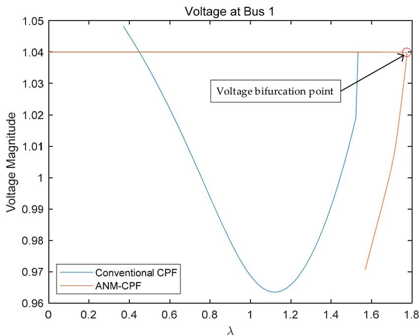
Figure 8. V-lambda curve of bus 1 when  $\mu = 10^{-7}$ .
