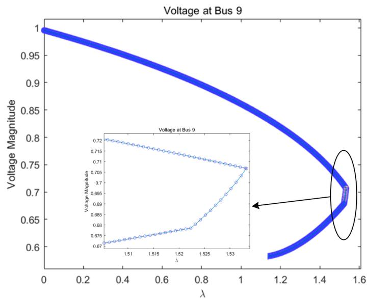
Figure 7. Step size  $s = 0.001$  for conventional predictor-corrector method.
