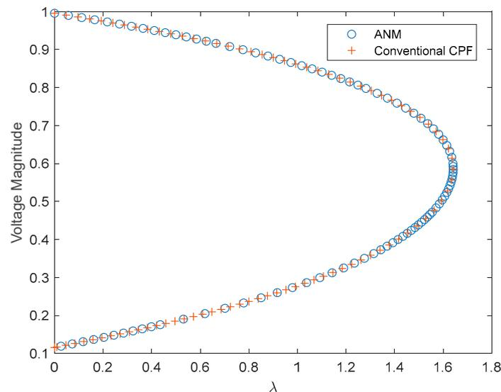
Figure 1. V-lambda curve of bus 9 for both methods.
