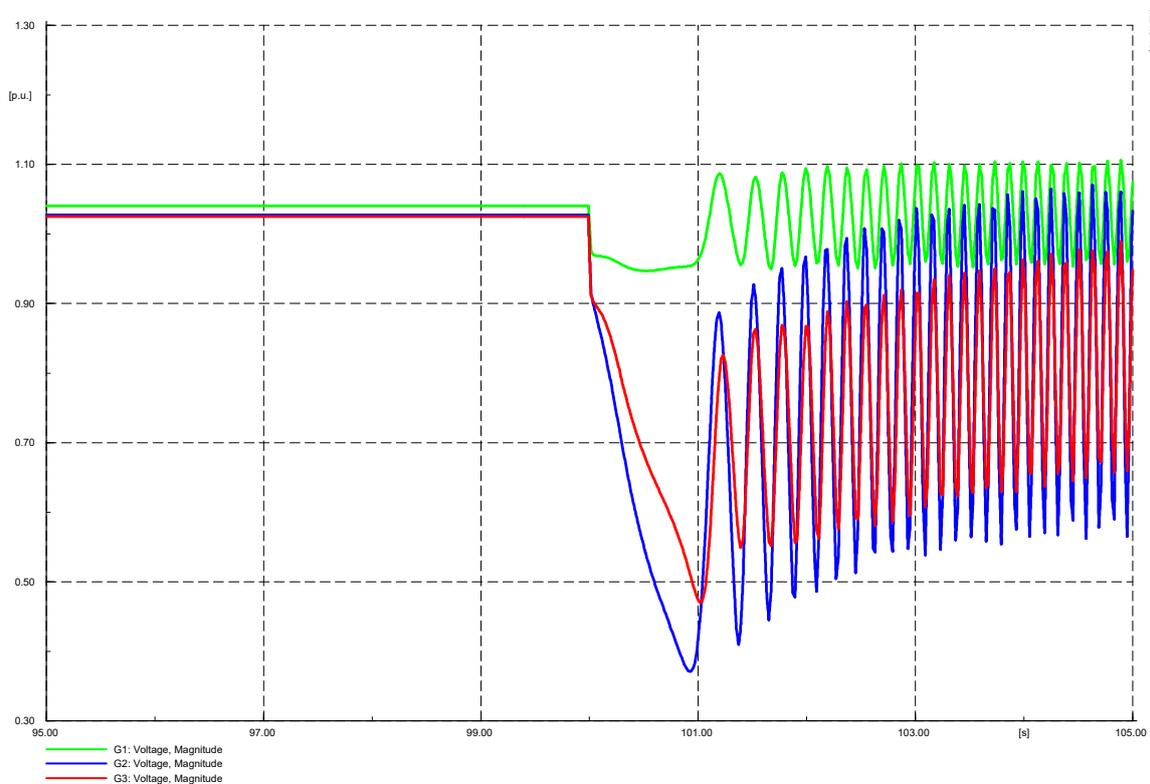
**Figure 2.** Voltage transient stability analysis results of bus 1, 2, and 3.
