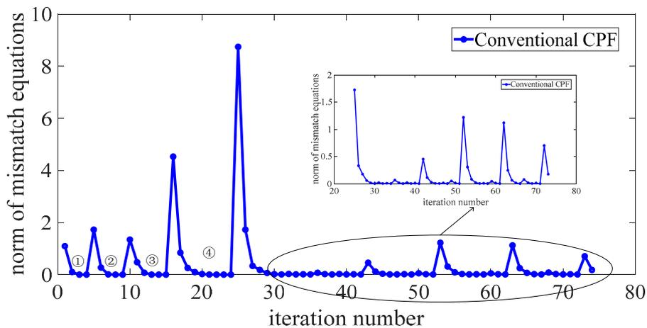
Figure 11. Conventional CPF corrector iteration at  $\lambda = 0.01$ .
