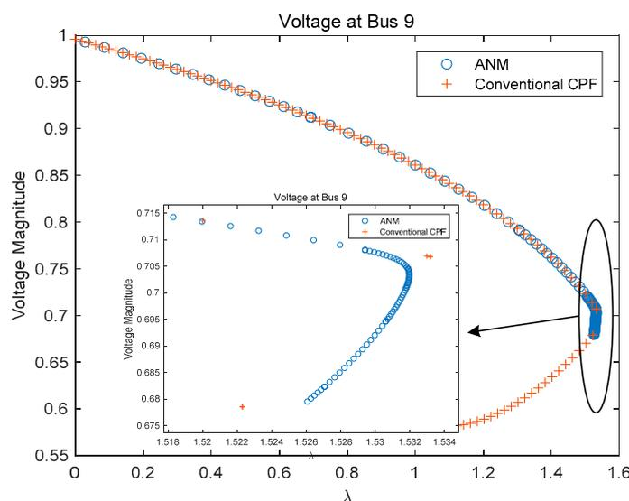
Figure 6. V-lambda curve of bus 9 for both methods.
